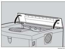
Holding the Mailbox on both sides, align the catches with the holes on the printer and insert.
